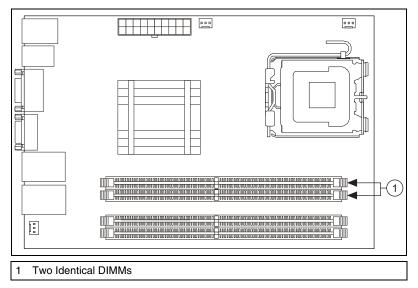
Figure B-19. Two Identical DIMMs in DIMM 1 and DIMM 2
